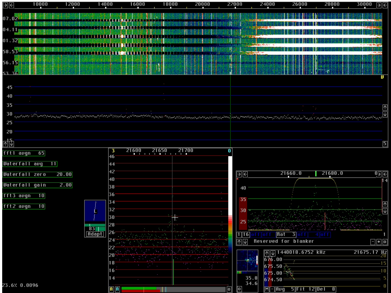
Figure 6. Linrad screen receiving Dave W5UN's EME signal at 21672 Hz. You can see Dave's signal beneath the cursor in the waterfall, main spectrum, high resolution spectrum, and baseband spectrum displays. In the baseband spectrum display you can see his keying sidebands within the yellow filter curve. To the right of the high resolution display the polarity display shows that Linrad is automatically controlling the polarization angle of the received signals and that Dave's polarization as received is nearly vertical, at 83 degrees. Additional details are given in the text.
